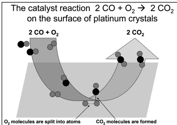
Structural model of the catalyst reaction
