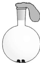
*Round flask filled with charcoal and closed with an air balloon*
