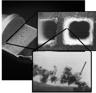
Electron microscopy image of the interior of a catalytic converter
